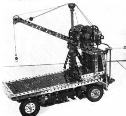
Well detailed Collis Crane Truck by Eric Jenkins. Power is provided to chassis via a differential. Crane luffing and hoisting by separate motor. All movements battery driven
