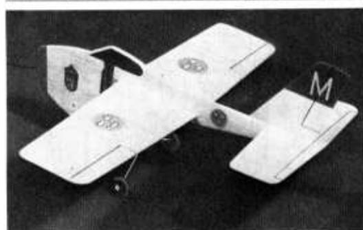
carefully warp up the rear edge of the tailplane in order to obtain extra height when flying. Your first test flight will reveal if this will be necessary.
