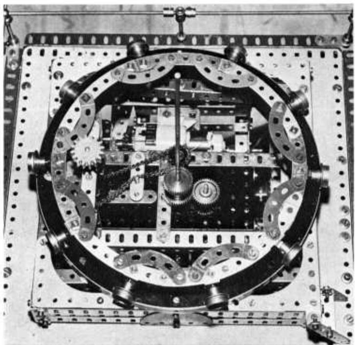
A high view of Mr. Evans' model, with jib removed, looking down into the supporting tower. Note the simple planetary gear arrangement which takes two drives up to the jib.
