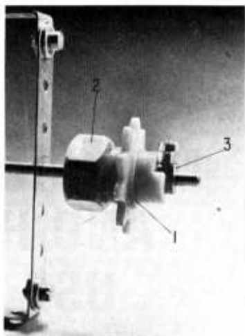
This picture illustrates a method of fixing a Plastic Meccano Sprocket Wheel to a "metal" Meccano Rod using Collars instead of a Coupling. Under operating conditions, the assembly would of course be mounted against the supporting framework.
