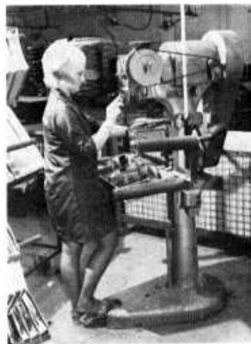
Riveting radiator-grille components on a B & TR Co. automatic-feed rivet-setting machine at the British Leyland (Austin Morris) factory at Cowley, Oxford.
