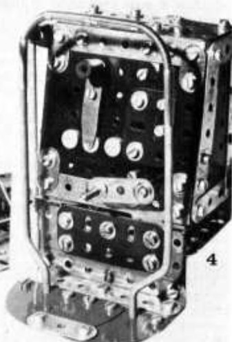
Fig. 1 Hornby transformer Type T20 for 20 volt locomotives with speed controller. Fig. 2 Similar transformer Type M20 for 20 volt Meccano A.C. D.C. motors such as E20R and E15R. Fig. 3 One way of making a two-way switch, mechanically operated, from Standard Meccano and Electrical parts. Fig. 4 Another two-way switch, hand-operated, also made from standard parts. Fig. 5 Meccano electrical parts used to make a neat distribution board on the control platform of a giant crane.
