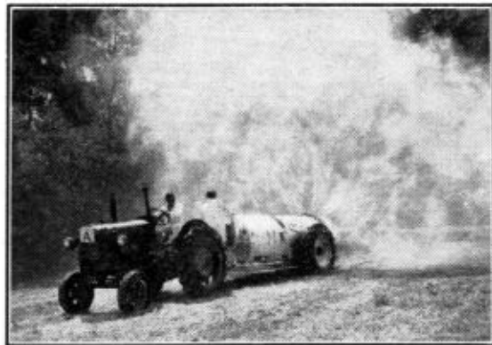
The Autoblaster at work. This powerful machine develops a 100 mile an hour blast into which spraying material is introduced. Photograph by courtesy of "Sport and Country."
