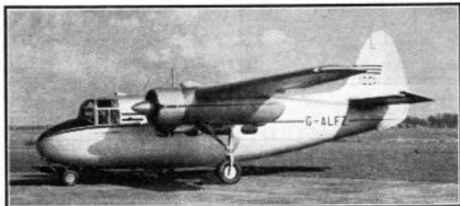
The Percival "Prince," a twin-engine 8-12 passenger transport. Photograph by courtesy of Percival Aircraft Ltd.
