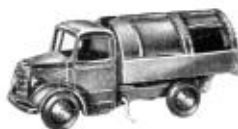
Bedford Refuse Wagon No. 25v Sliding covers, tipping mechanism, opening rear door
