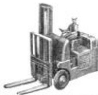
Coventry Climax Fork Lift Truck, No. 14c The loading carriage is raised by turning a handle.
