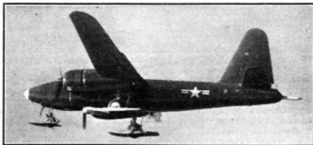
With ski-gear extended for landing, the U.S. Navy's specially equipped Lockheed "Neptune" makes its first test flight. Photograph by courtesy of Lockheed Aircraft Corporation.
