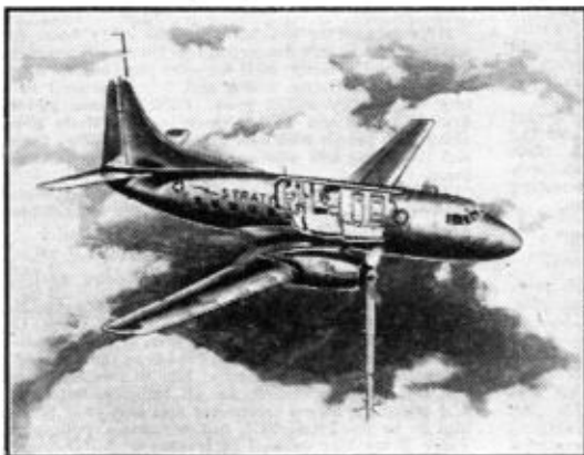
Cutaway view of Martin 2-0-2 air liner showing how television and broadcasting equipment would be installed for high-altitude transmitting of programmes.
