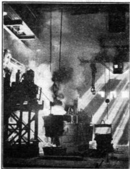
Pouring steel from an arc furnace into a ladle in readiness for ingot making. The illustrations in this article are reproduced by courtesy of Thomas Firth and John Brown Ltd., Sheffield.
