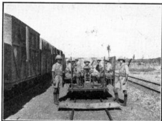
An armoured pump-handle type trolley, with the protective plating removed at one end to show how the crew are accommodated.
