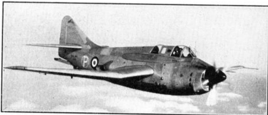
Fairey 17 anti-submarine patrol-bomber, first aircraft to fly powered by a coupled "propjet" engine. Photograph by courtesy of The Fairey Aviation Co. Ltd.
