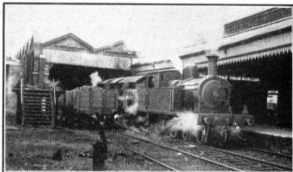
B. and C.D.R. No. 15, one of the 4-4-2 tanks ready to leave Downpatrick on the 12.5 p.m. for Ardglass.
