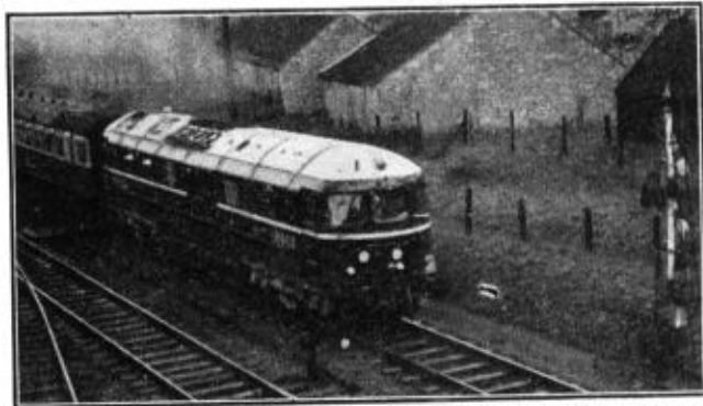
B.R. 18000, the first gas-turbine locomotive in Britain, passing Bathampton on a trial run between Paddington and Bristol. Photograph by A. F. Wright.
