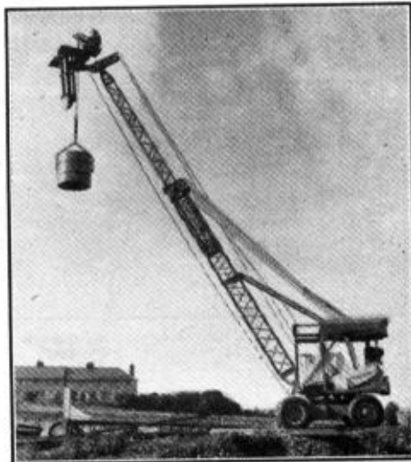
A specially equipped mobile crane designed for speeding up the harvesting of palm nuts. Photograph by courtesy of R. H. Neal and Co. Ltd., Ealing.
